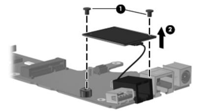
4. Remove the modem module, cable, adhesive tape, and RJ-ll port.
